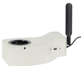
Dovetail mount with built-in 0.43X relay lens
