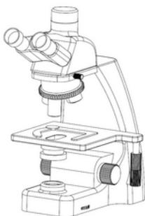
1 Trinocular Microscope
